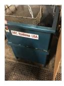
The parts are dipped and allowed to fully coat all exposed surfaces, then raised and allowed to drip dry. After five minutes, the film is cured and the part is ready to go into storage on the shelf. The customer began dipping parts in November, 2015 and fifteen (15) months later, they are still receiving full protection and are rust free.
